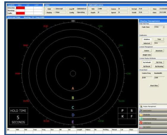
Fig 2 – Fusion POLAR Window Synthetic Contacts are scaled (in frequency or amplitude) and displayed via the Plan Position Indicator (PPI) Window
